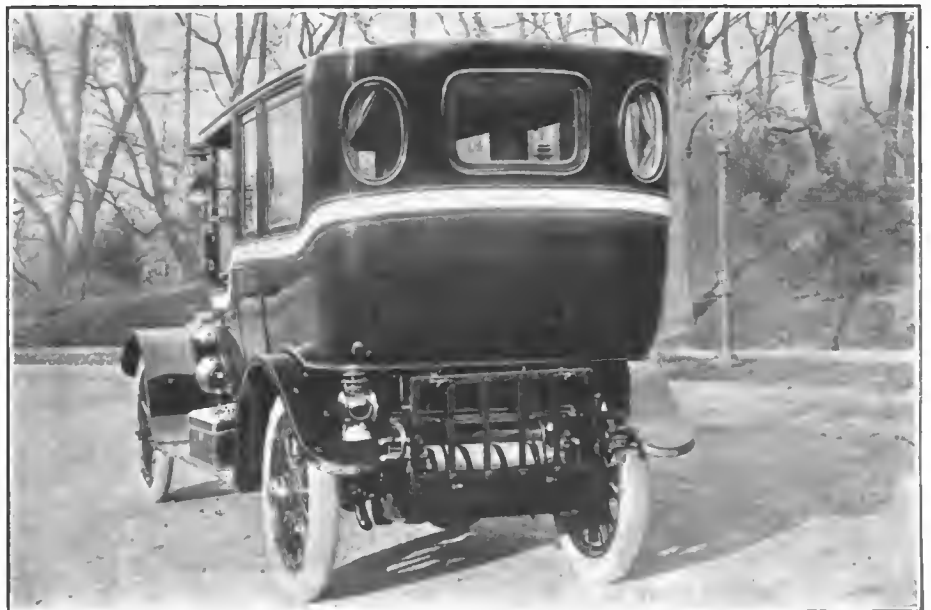
View of 1912 Alco limousine, showing new marine windows in rear
